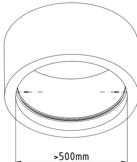
4. Solder power cable to strip, clean the profile surface with alcohol to have it fat and dust free. Insert Flex Strip into profile.
